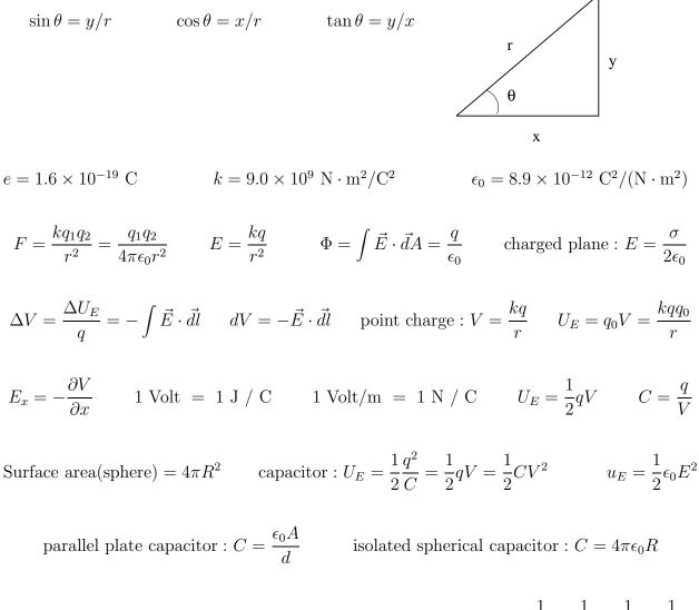
capacitors in parallel :  $C = C_1 + C_2 + C_3...$  capacitors in series :  $\frac{1}{C} = \frac{1}{C_1} + \frac{1}{C_2} + \frac{1}{C_3}...$
